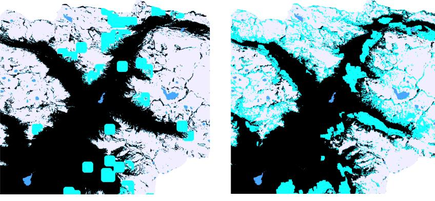
A cloud-filling temporal interpolation process is performed separately for Landsat 8 and Sentinel 2 and for MODIS.
